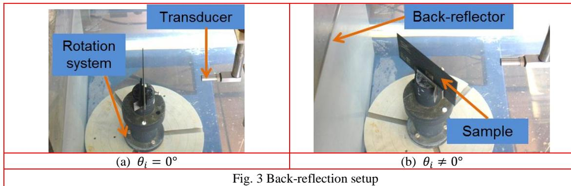
Fig. 3 Back-reflection setup
