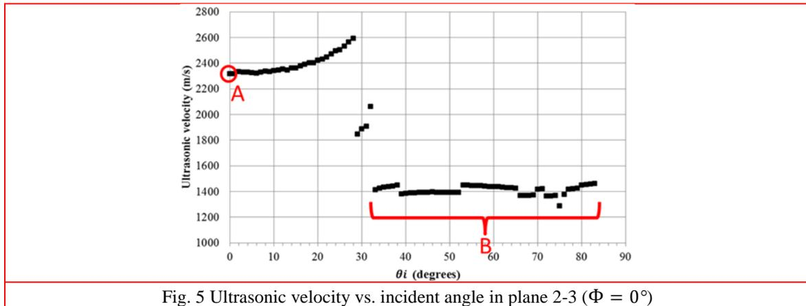
Fig. 5 Ultrasonic velocity vs. incident angle in plane 2-3 ( $\Phi = 0^\circ$ )
