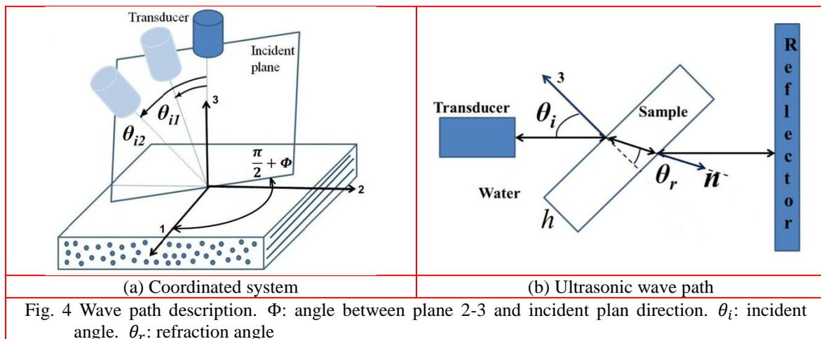
Fig. 4 Wave path description.  $\Phi$ : angle between plane 2-3 and incident plan direction.  $\theta_i$ : incident angle.  $\theta_r$ : refraction angle
