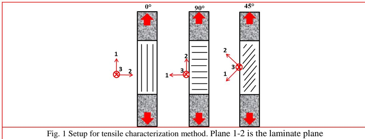
Fig. 1 Setup for tensile characterization method. Plane 1-2 is the laminate plane
