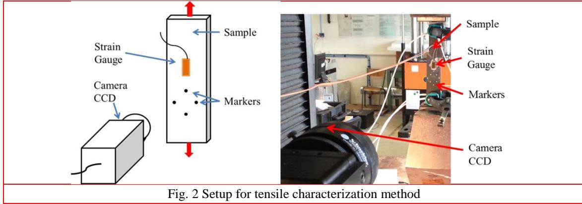
Fig. 2 Setup for tensile characterization method
