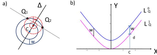
**Fig. 5.** a) The 2D annulus having  $Q_1$  and  $Q_2$  as border point has its centers on the bisector  $\Delta$  of the line segment  $Q_1Q_2$ . b) All annuli for which  $Q_1$  and  $Q_2$  are on  $B_e$  correspond to the set of all the vertical line segments of length  $\omega$  having one of its endpoints on  $L_Q^0$  and the other on  $L_Q^1$ .
