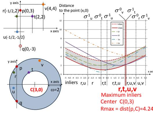
**Fig. 7.** 2D example: six points  $p=Q_1$ ,  $q=Q_2$ ,  $r$ ,  $u$ ,  $v$ , and  $t$  in the primal space and their corresponding curves. The maximum number of inliers for an annulus having  $p$  and  $q$  on  $B_e$  is reached when the center has an  $x$ -value around 3.
