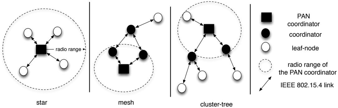
Fig. 2. The different topologies proposed in IEEE 802.15.4
