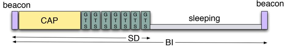
Fig. 1. Superframe structure of IEEE 802.15.4
