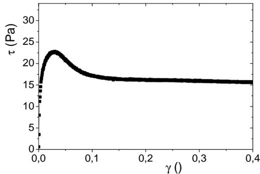
Figure 3: Characterization of the suspending paste: stress as a function of strain obtained for the static yield stress measurement; a shear rate of  $0.01 \text{ s}^{-1}$  is applied to the sample after a rest of 4 min.
