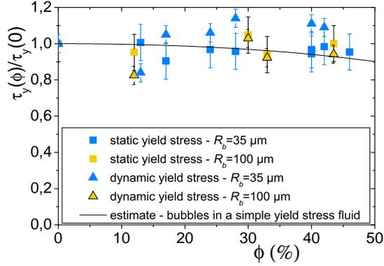
Figure 6: Dimensionless yield stress (static:  $\square$ , and dynamic:  $\triangle$ ) as a function of the gas volume fraction, for the two series of suspensions studied. The full line is a micro-mechanical estimate for the dimensionless static yield stress of suspensions of monodisperse bubbles in model yield stress fluids (Ducloué et al., 2015).
