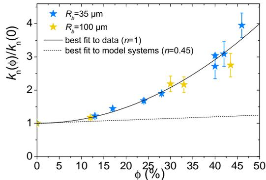
Figure 8: Dimensionless plastic viscosity of the two series of suspensions of bubbles in the metakaolin paste ( $n = 1$ ), as a function of the gas volume fraction. The full line is a phenomenological best fit to the data. The dashed line is a best fit to data obtained on suspensions of bubbles in model yield stress fluids with  $n = 0.45$ .
