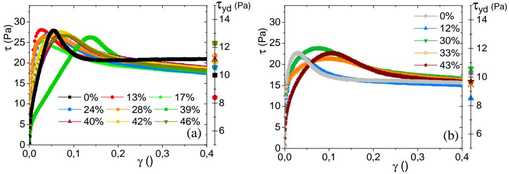
Figure 5: Stress as a function of strain during the static yield stress measurement on suspensions of (a):  $R_b = 35\mu\text{m}$  and (b):  $R_b = 100\mu\text{m}$  bubbles in the metakaolin paste. A shear rate of  $0.01\text{ s}^{-1}$  is applied to the samples after a 4 minute rest. The dynamic yield stress of the same samples, obtained from the flow curves, is plotted on the right axis.
