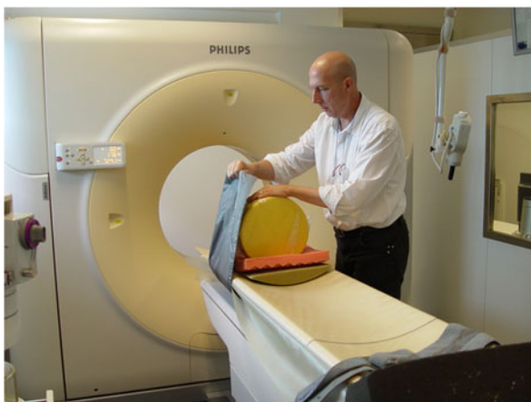
Fig. 1 CT scanner (Philips CT Brilliance 16P with cheese and operator)
