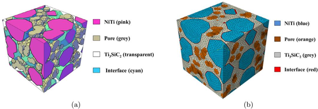
Fig. 18: Detailed 3D, multiphase (a) numerical microstructure and (b) finite element mesh used for the thermal analysis of a NiTi –  $\text{Ti}_3\text{SiC}_2$  composite. Reprinted from [93] with permission from Elsevier.
