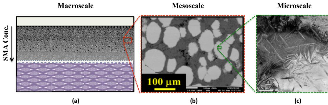
Fig. 10: Multiple scales of interest in the analysis of SMA composite materials: (a) *Macroscale* – A functionally graded, hybrid composite for extreme environments<sup>2</sup>; (b) *Mesoscale* – A NiTi (white gray)  $\text{Ti}_2\text{AlC}$  (darker gray) with heterogeneous microstructure, porosity (black), and reaction layers (Reprinted from [187] with permission from Elsevier); and (c) *Microscale* – Martensitic twins and accompanying nanoprecipitates of a NiTi<sup>3</sup>.
