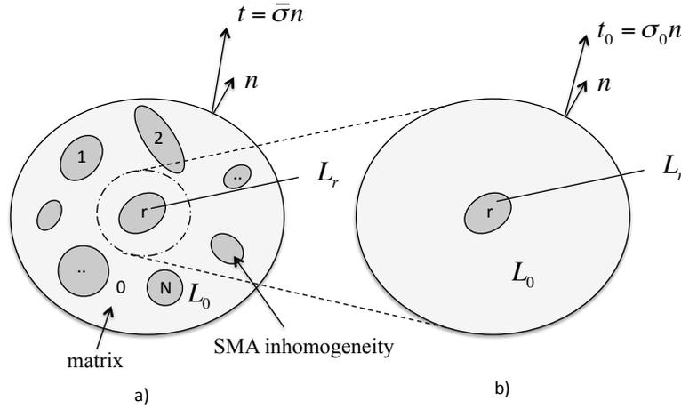
Fig. 12: Illustration of the boundary value problem considered for analysis via Eshelby-based mean field approaches: (a) a composite comprised of  $N$  distinct, ellipsoidal inhomogeneity phases embedded in a distinct matrix and (b) the Mori-Tanaka problem for the  $r$ -th phase. ©IOP Publishing. Reproduced from [252] by permission of IOP Publishing. All rights reserved.
