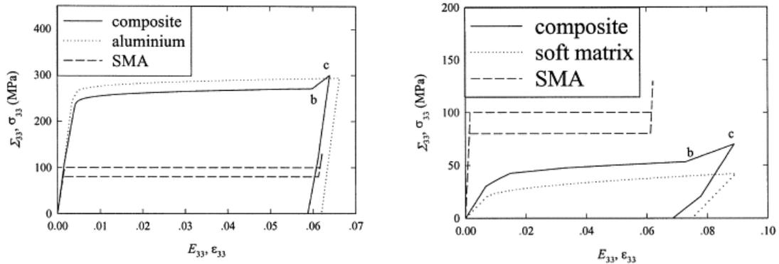
(a) The axial stress strain curves of composite, aluminium and SMA under uniaxial tension.
