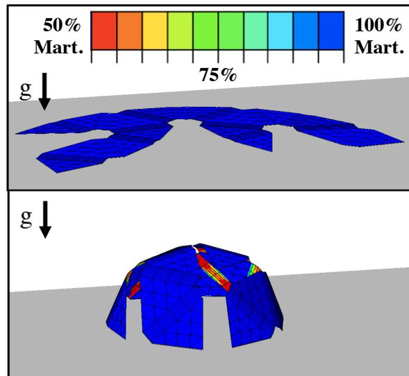
Fig. 20: Initial and final configuration of a reconfigurable SMA composite. Selected heating of pre-strained wires from the initial configuration is used to selectively transform the material and induce the deformations necessary to produce the final shape. Reprinted from [351] with permission from Elsevier.
