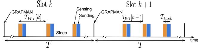
Fig. 1: Dynamic adaptation of the wake up interval.
