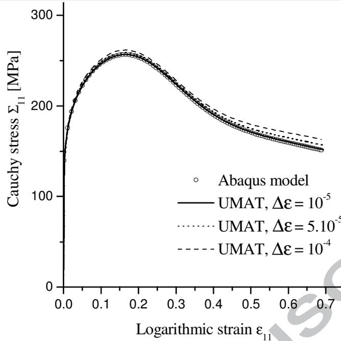
**Fig. 1.** Comparison between the Abaqus model (implicit time integration scheme) and the developed explicit UMAT subroutine (using three different-sized strain increments) for a uniaxial tensile test performed on a material similar to the Al5182 aluminum alloy.
