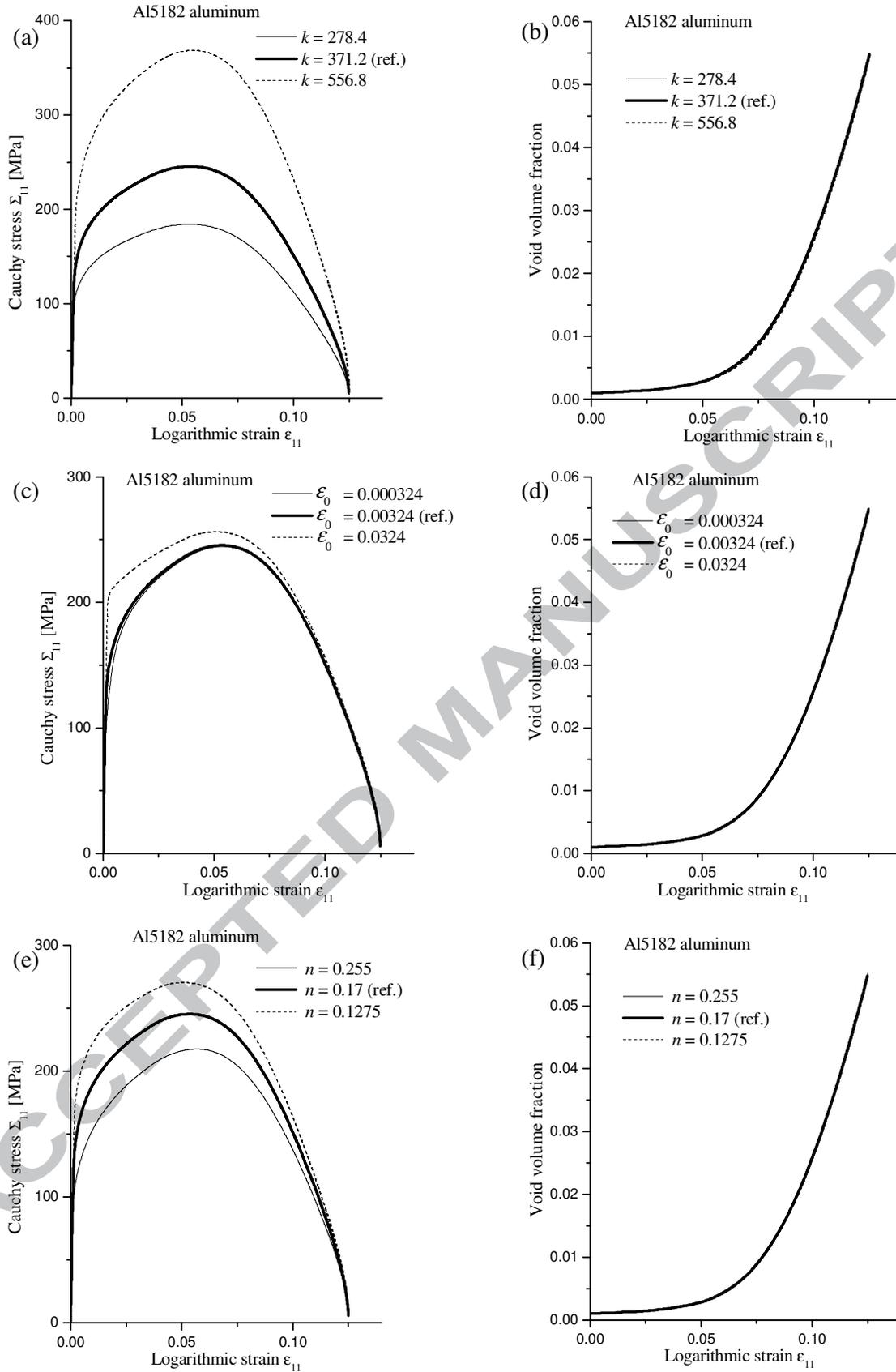
**Fig. 16.** Evolution of the Cauchy stress and void volume fraction until localization along the BBT strain path when the parameters  $k$ ,  $\epsilon_0$  and  $n$  are varied for the Al5182 aluminum alloy.
