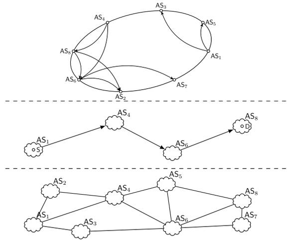
Figure 1. Network layers of our proposal. The first layer corresponds to the existing links between the ASes, the second one to the chosen path  $\prec S, D \succ$ . The final layer corresponds to the DHT organizing the score managers of ASes;  $AS_8$  and  $AS_6$  are the score managers of  $AS_4$ , etc.
