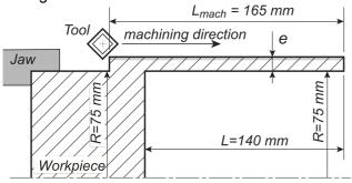
Figure 3: Section of the machined tube
