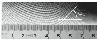
Figure 6: Chatter zone and wavelet slope
