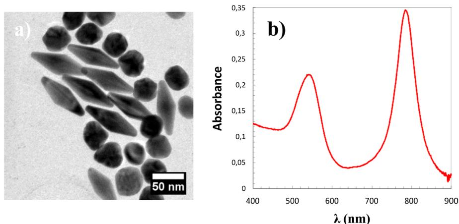
**Figure 1.** (a) TEM image of Au bipyramids synthesized by addition of 60  $\mu\text{L}$  of seed solution into growth solution including 5-bromosalicylic acid ( $\text{AR} \approx 2.7$ ) (Table S1, no. 3 experimental conditions detailed in Supporting Information, section 1-ii) and (b) corresponding UV-vis spectra of the solution.
