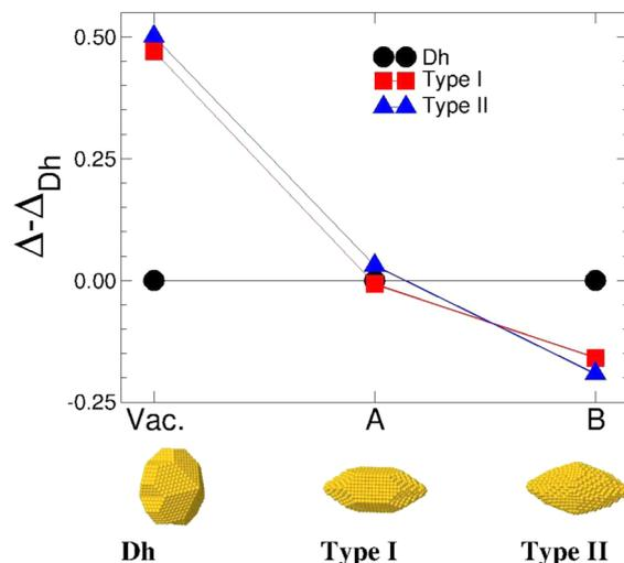
**Figure 6.** (top) Excess surface energies of the most stable elongated pentatwinned gold particles with respect to the isotropic decahedral (i-Dh) ones  $\Delta - \Delta_{\text{Dh}}$  (eV/N<sup>2/3</sup>). (bottom) i-Dh, type I, and type II particles corresponding, respectively, to the most stable structures in vacuum and environments A and B, created with an average of 3000 gold atoms per particle.
