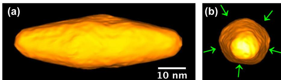
**Figure 4.** (a) Figure e-tomo 3D volume of a bipyramid obtained from a DART reconstruction procedure and (b) the bipyramid viewed along the elongation direction. A clear pentagonal section is evidenced.
