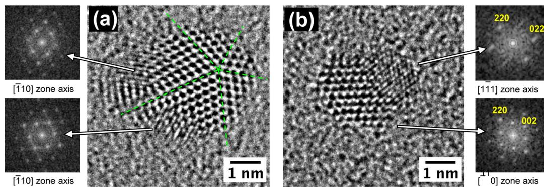
**Figure 5.** Structural analysis of twinned seeds. (a) Ultra-HRTEM image of a 3.3 nm particle with FFT analysis of selected areas. (b) Ultra-HRTEM image of a 2.7 nm seed particle with different orientation.
