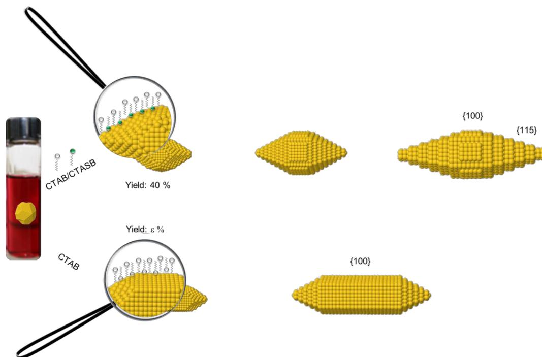
**Figure 7.** Formation mechanism of bipyramids and nanorods. In the present case, the bipyramids are formed by a silver(I)-assisted process in CTAB solution and deduced from HRTEM; pentatwinned structure is maintained along the growth. For pentatwinned nanorod formation, they are obtained without silver from decahedra seeds in a very low yield.
