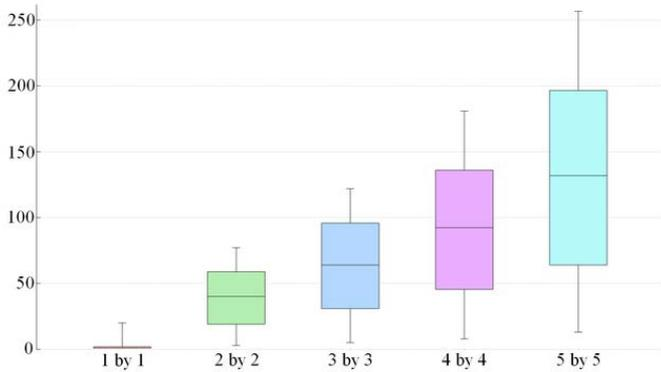
Fig. 6. UPnP device startup time in milliseconds
