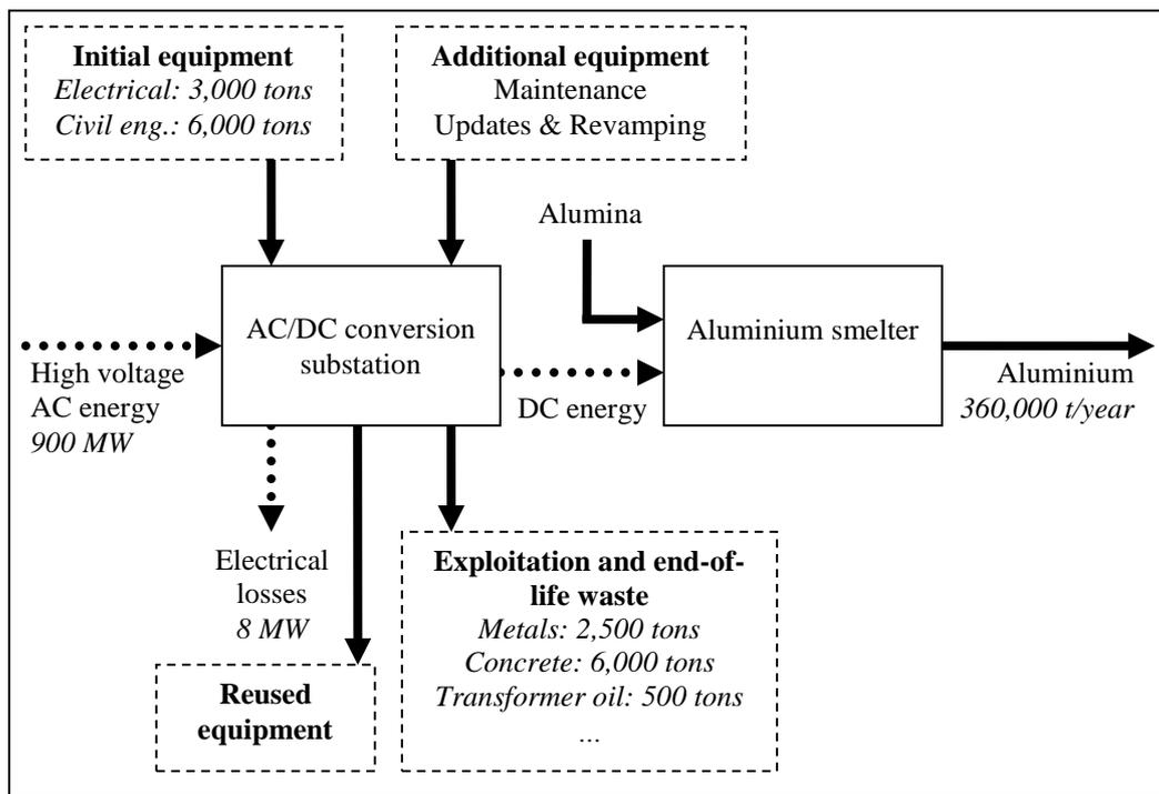
**Figure 6. Overview of the flows associated with a substation life cycle. (Figures rounded off for confidentiality reasons)**
