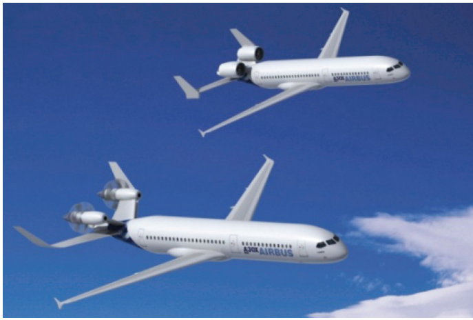
Figure 23 - Airbus views on a futuristic design for 2030 : rearward engines with or without Open Rotors (left) and embedded engines (right).
