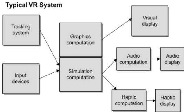
**Figure 2. Components of a typical VR system [10]**
