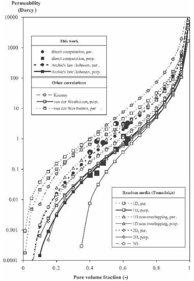
FIG. 8. Permeability estimates: comparison of direct computations from CMT images and established models.
