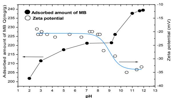
Fig. 1. Influence of the pH of stevensite-MB aqueous dispersions on the MB amount adsorbed onto stevensite and zeta potential.
