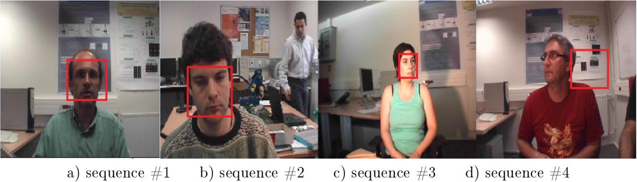
Figure 5: Rectangular bounding box  $BB$  produced by the VJ face detector in various sequences: a), b), c) correct detections; d) false detection.
