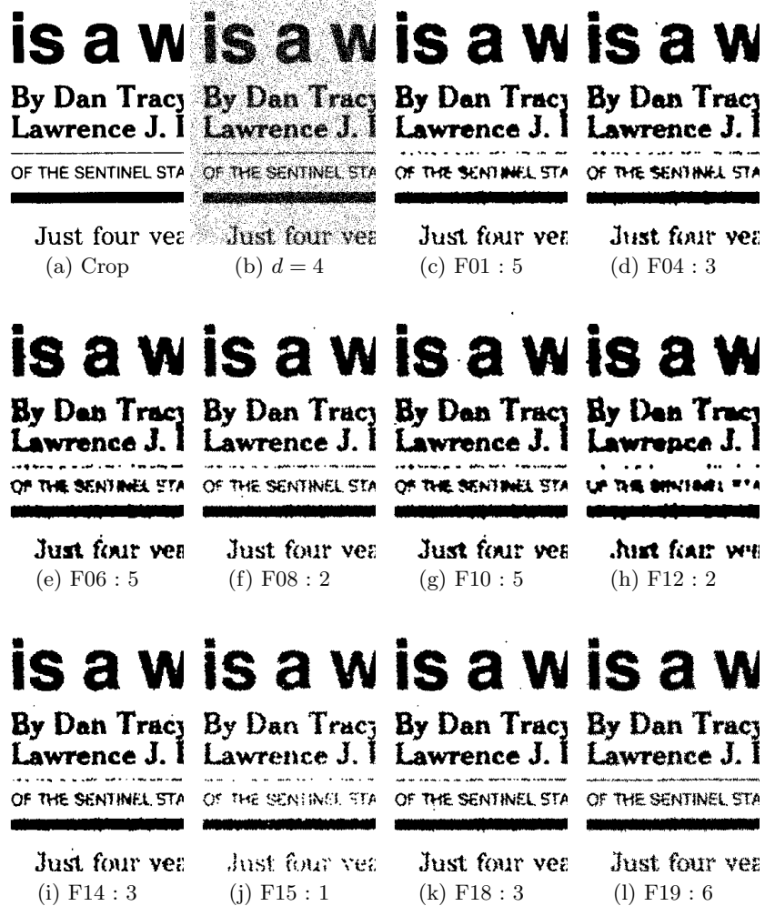
Fig. 3: First test protocol sample on binary documents. Original and degraded images with binary degradation model, along with best filtering results obtained on image 3b, under the form [ID : f ].
