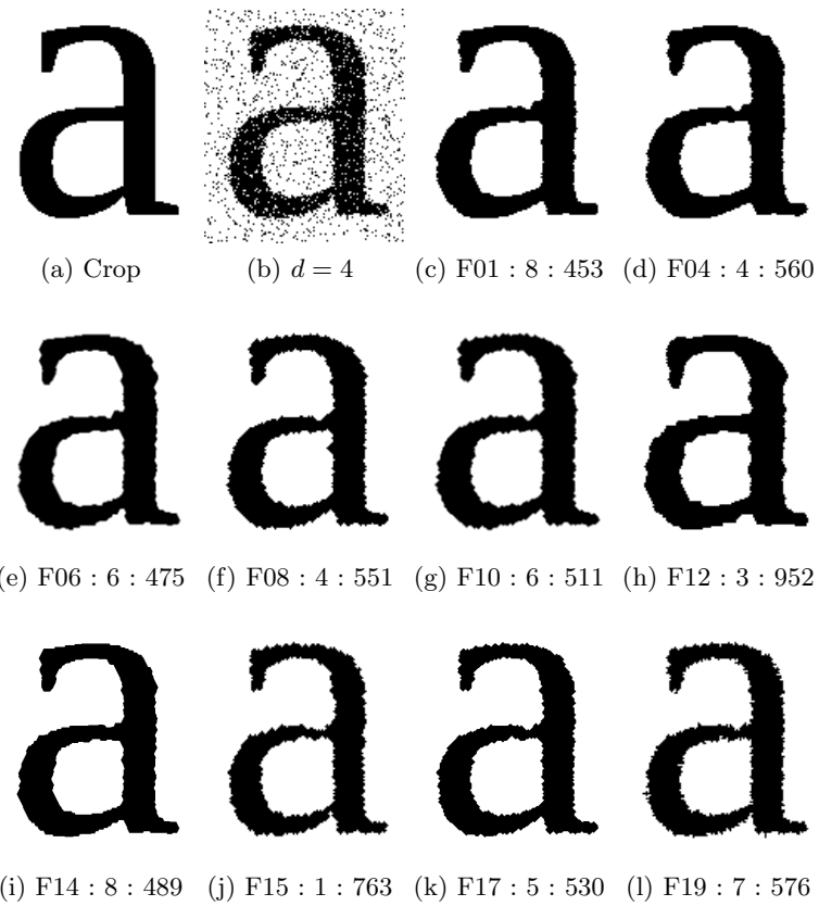
Fig. 4: Second test protocol sample on a binary document. Original and degraded images with binary degradation model, along with best filtering results obtained on image 4b ( d = 4 ), under the form [ID : f : MSE].
