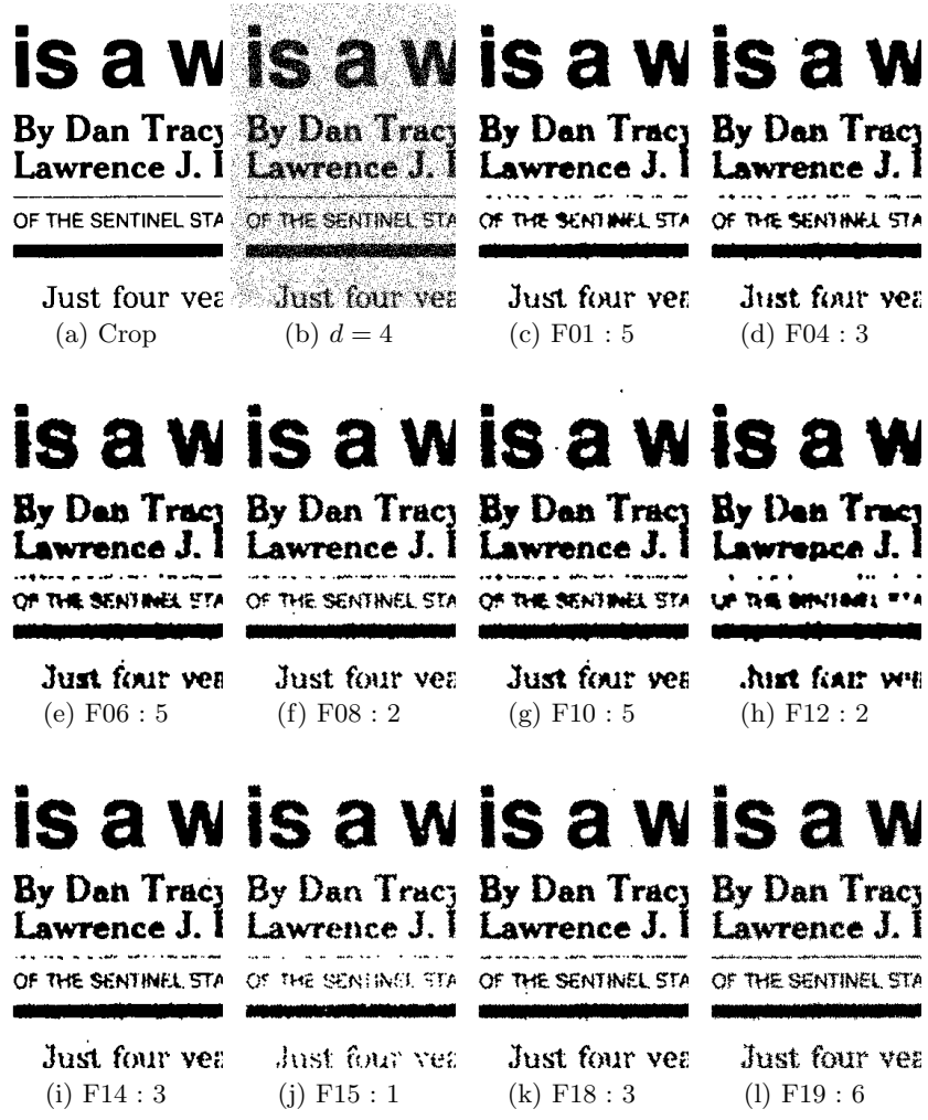
Fig. 3: First test protocol sample on binary documents. Original and degraded images with binary degradation model, along with best filtering results obtained on image 3b, under the form [ID : f ].
