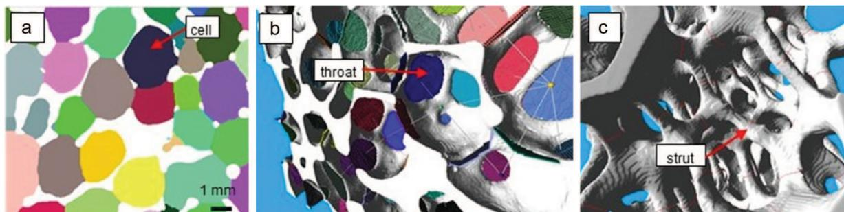
Fig. 5. (a) Segmentation of each cell on a 2D view, (b) segmentation of each throat and connectivity calculation on a 3D view, (c) strut size calculations on a 3D view. (For interpretation of the references to color in the text, the reader is referred to the web version of this article.)
