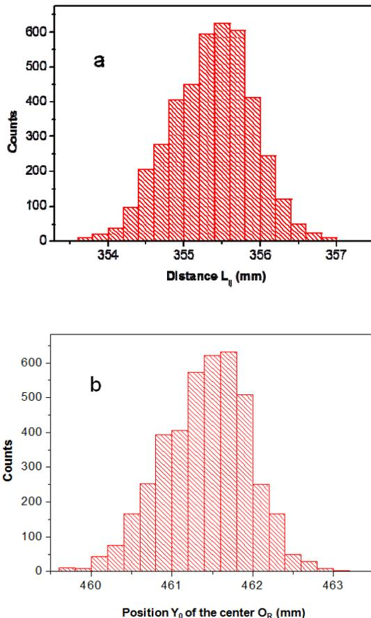
Fig. 3. Histograms. *a*: dispersion of a static distance on a set of 4200 measurements; *b*: consequence on the dispersion of the position of the centre of the set of axes. Standard deviation is 0.53 mm for each.
