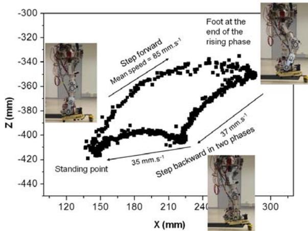
Fig. 10. Plot of the projection in the vertical plane  $(X, Z)$  of the stride movement composed of three phases. Three photographs show the main points: the standing point, the end of the rising step and the mid-point of the return. One can see that the motion is quite small and that it is important to have a good resolution.
