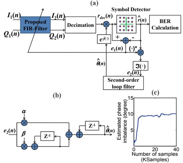
Fig. 4. (a) Schematic of DSP blocks for the received samples. (b) Second-order loop filter structure. (c) Convergence of the estimated phase imbalance.
