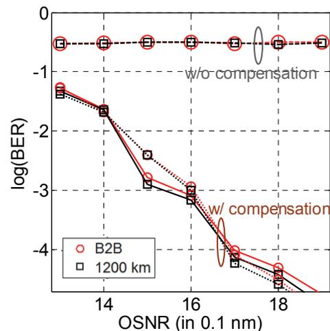
Fig. 7. BER versus OSNR under the impacts of chromatic dispersion and IQ imbalance. Solid lines: no IQ imbalance and with compensation. Dotted lines: with IQ imbalance of  $20^\circ$  and with compensation. Dashed lines: with IQ imbalance of  $20^\circ$  and without compensation.
