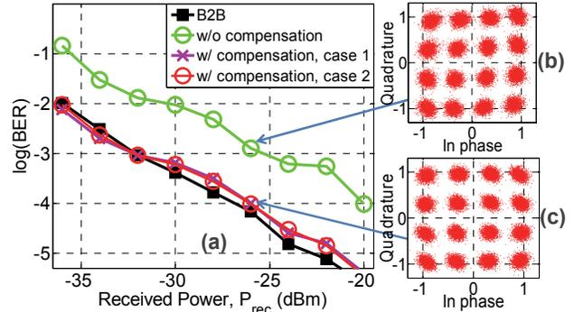
Fig. 5. BER versus received power for 10° phase imbalance.
