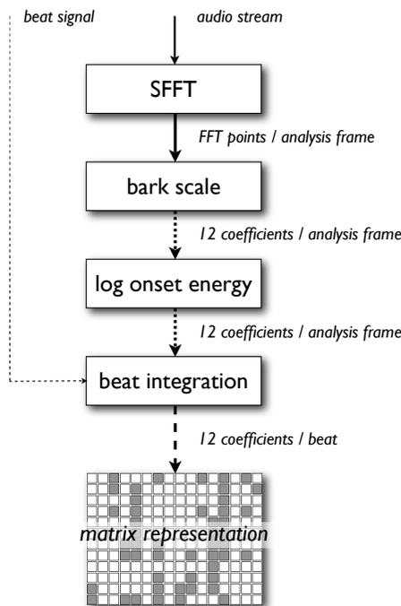
Figure 2: Data-flow diagram of the *X-Micks/Ma-Tricks* analysis stage
