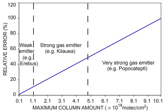
Figure 8: Relative error on the approximation of the mean  $\text{SO}_2$  column amount ( $\overline{CA}$ ) along the different directions in the wide field of view by the  $\text{SO}_2$  column amount measured with the DW-FOV DOAS ( $CA_{WFOV}$ ), according to Eq. A.18 (for more explanations, see Appendix A). For calculations, an averaged value of the  $\text{SO}_2$  cross section, estimated over the wavelength range used for fit, is considered ( $10^{-19}$  cm<sup>2</sup>).
