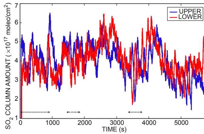
Figure 2: Time-series of SO<sub>2</sub> column amounts for both upper (blue) and lower (red) wide field of view spectrometers at Erebus on 26 December 2006 from ~20:24 h to 22:02 h *UTC*. Dashed lines show periods of time when a bend was observable in the plume at a height less than 200 m above the crater, i.e., below the altitude of the upper spectrometer's FOV.
