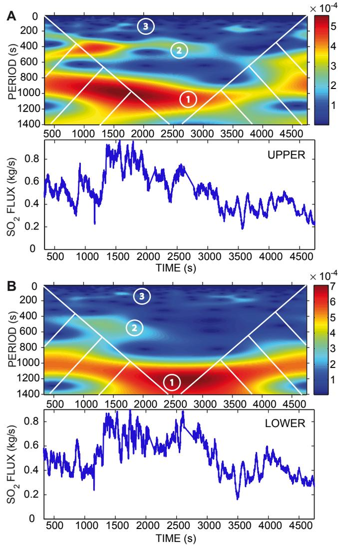
Figure 6: Wavelet transform (modulus) and time-series of SO<sub>2</sub> fluxes (in kg s<sup>-1</sup>) for (a) upper and (b) lower spectrometers. Note that flux time-series are linearly interpolated to fill the few data gaps described in Fig. 5. The three populations of distinctive periods present in the signal (referenced as Patterns 1,2,3 in the figure) are discussed in the text. The cone of influence (white lines) delimits cross-hatched regions, inside which edge effects are non-negligible.
