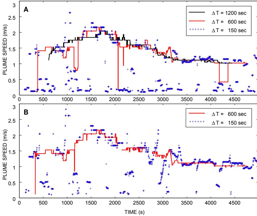
Figure 3: Plume speed *vs.* time since start of the dataset start at 20:24:48 UTC for (a) different sliding windows used for correlation analysis (with a duration  $\Delta T$  of respectively 1200, 600 and 150 s), (b) a narrow and long sliding window ( $\Delta T = 150$  and 600 s), using the criterion selecting the first local maximum in the CCF function, relative to the time shift, with an amplitude above a threshold of 0.5.
