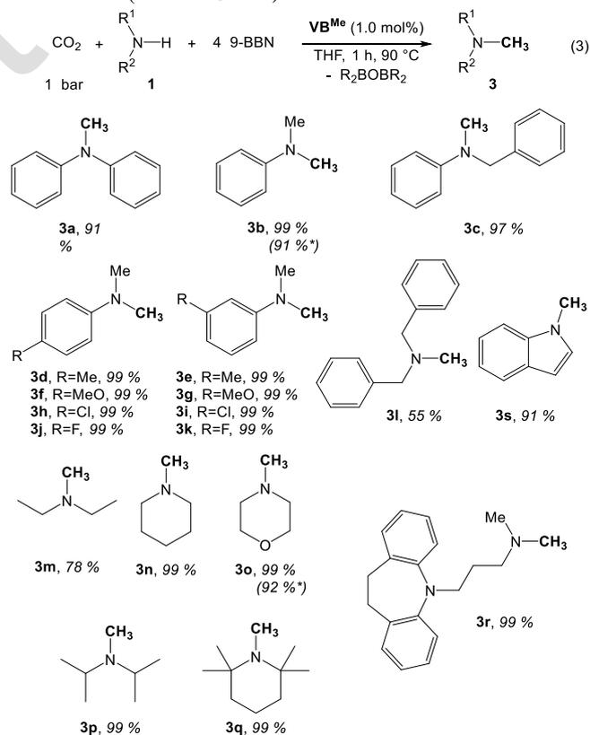
**Scheme 2.** Metal-free catalytic methylation of secondary amines with CO<sub>2</sub> and 9-BBN. Reaction conditions: amine (0.20 mmol), hydroborane (0.80 mmol), **VB<sup>Me</sup>** (0.002 mmol), THF (0.50 mL), CO<sub>2</sub> (1 bar); yield determined by GC/MS using mesitylene as an internal standard, after calibration. (\*Isolated yield)
