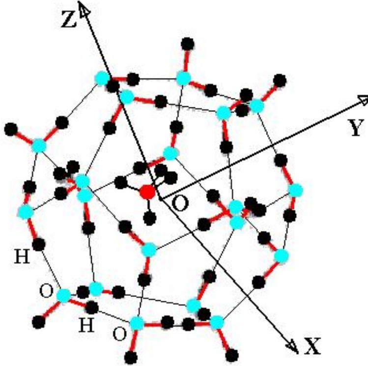
Figure 1: Trapping geometry of a guest molecule ( $\text{CH}_4$  for instance) in a small cage of the structure type I.  $(O, X, Y, Z)$  represents the absolute frame tied to the clathrate lattice.
