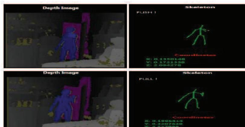
Figure 4: Recognition of push and pull gesture
