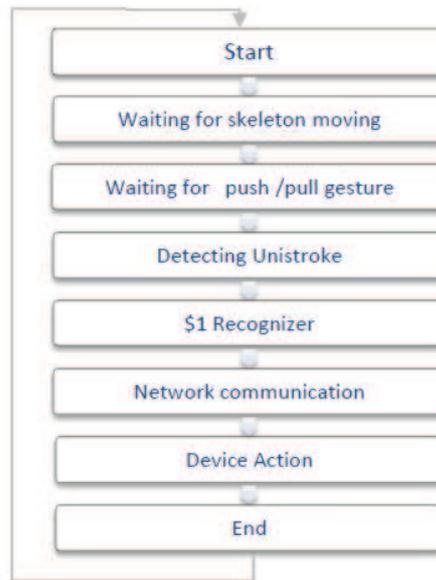
**Figure 5: Diagram of gesture recognition using Kinect**
