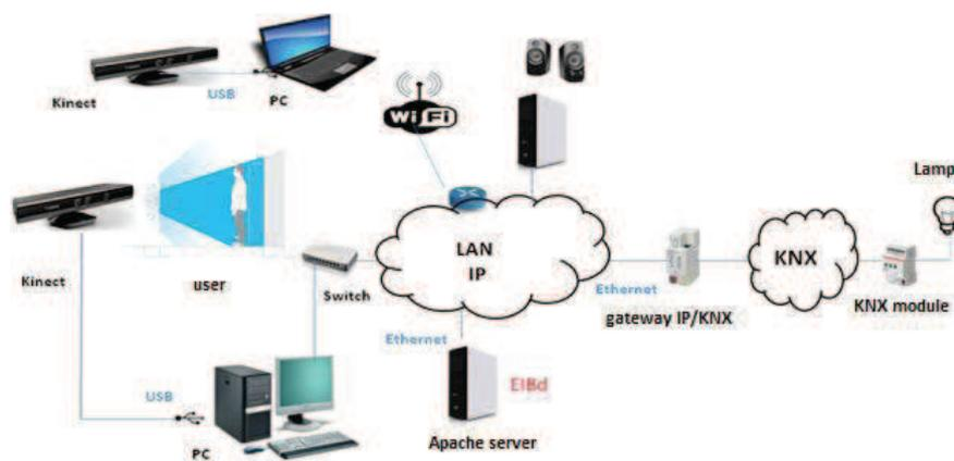
Figure 7: Network Interconnection IP/KNX
