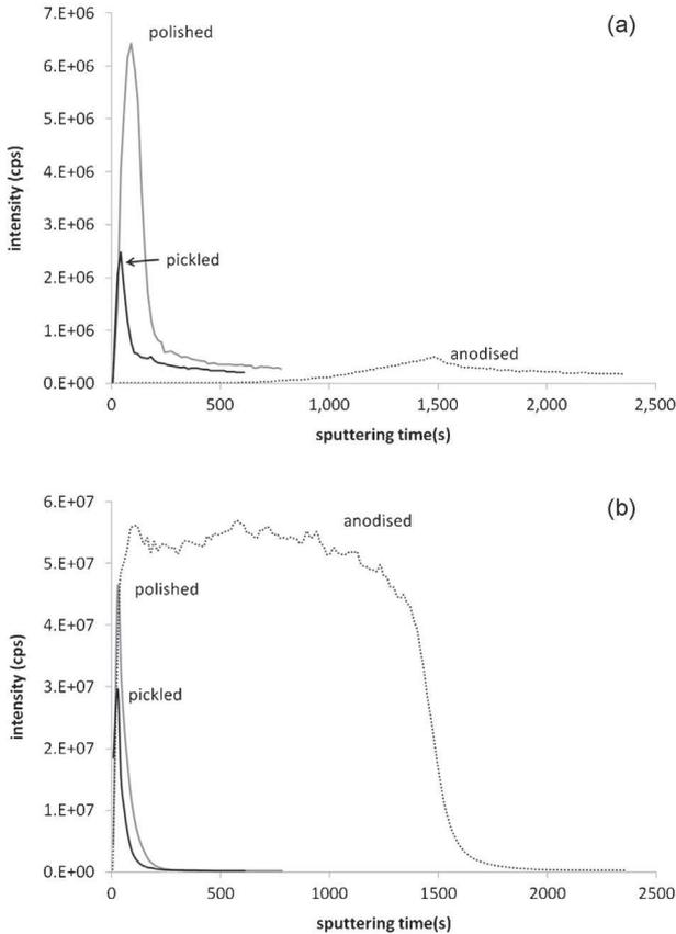
**Fig. 3.** (a) Hydrogen and (b) oxygen SIMS profiles obtained on rolled sample after three different steps: polishing then pickling (HNO<sub>3</sub>–HF (20–2 w%) solution, 20 °C, 200 s) and finally anodization (80 V, 1 M H<sub>2</sub>SO<sub>4</sub>, 20 °C, 2 min).
