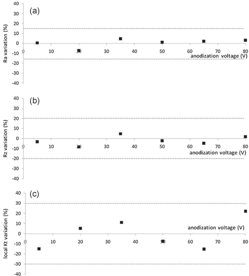
**Fig. 7.** Changes of (a)  $R_a$  (b)  $R_z$  average roughness values and (c) local  $K_t$  values as a function of the anodization voltage (5–80 V), i.e. the thickness of the film (16–195 nm) prepared on rolled sample pickled ( $\text{HNO}_3$ –HF (20–2 w%) solution, 20 °C, 200 s) then anodized (1 M  $\text{H}_2\text{SO}_4$ , 20 °C, 2 min). The dotted lines correspond to standard deviation.
