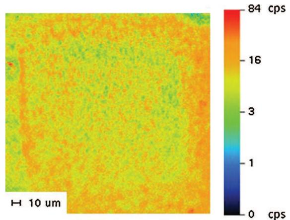
**Fig. 4.** SIMS surface mapping of hydrogen on a polished and then pickled sample (HNO<sub>3</sub>–HF (20–2 w%) solution, 20 °C, 200 s). In the middle of the sample appears a sputtered crater a few microns in depth.
