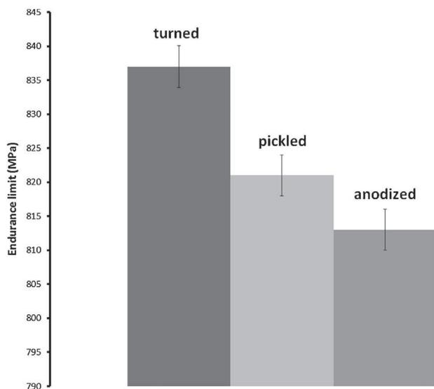
**Fig. 10.** Endurance limit of three samples: turned, turned then pickled ( $\text{HNO}_3$ -HF (20-2 w%) solution, 20 °C, 200 s), turned, pickled and finally anodized at 80 V (1 M  $\text{H}_2\text{SO}_4$ , 20 °C, 2 min).
