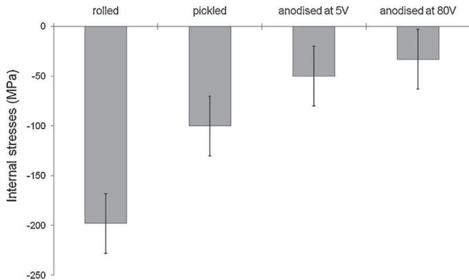
**Fig. 9.** Evolution of internal stresses obtained on four rolled samples after different surface treatments: rolled, rolled then pickled ( $\text{HNO}_3$ -HF (20-2 w%) solution, 20 °C, 200 s), rolled then pickled and finally anodized at 5 V (1 M  $\text{H}_2\text{SO}_4$ , 20 °C, 2 min) and a rolled then pickled and finally anodized at 80 V (1 M  $\text{H}_2\text{SO}_4$ , 20 °C, 2 min).
