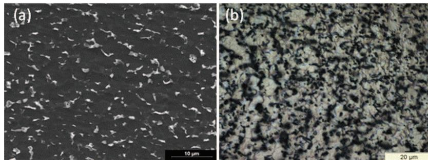
Fig. 1. (a) SEM view and (b) OM view of rolled sheet microstructure, previously pickled in a mixed 4 w% HF–3 w%  $\text{HNO}_3$  solution for 10 s at ambient temperature.
