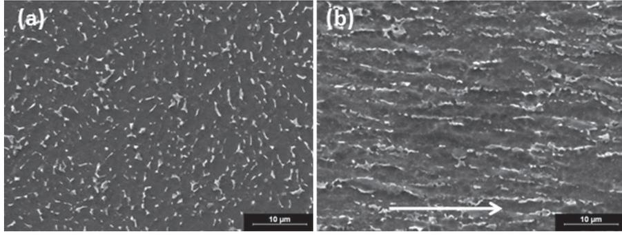
**Fig. 2.** SEM views (a) in radial direction and (b) in longitudinal direction (arrow) of forged bar microstructure, previously pickled in a mixed 4 w%HF–3 w%HNO<sub>3</sub> solution for 10 s at ambient temperature.
