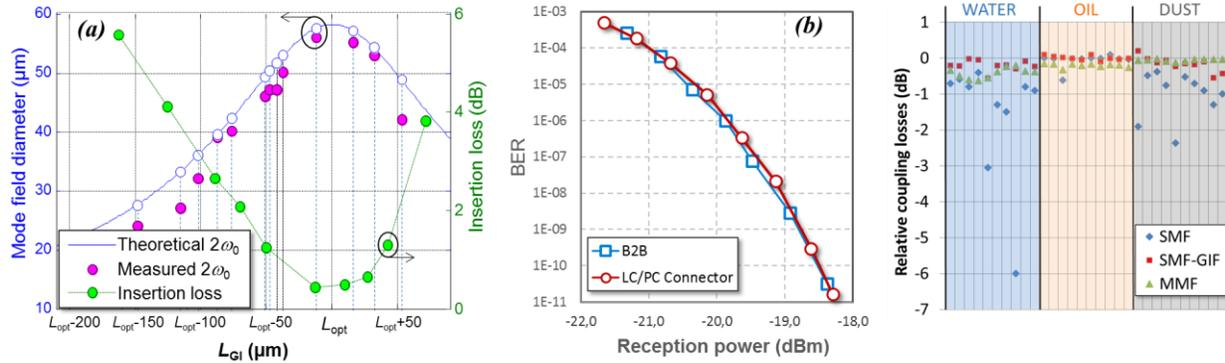
**Fig. 2.** (a) measurement of insertion losses, and beam waist of SMF-GIF LC/PC connectors, (b) BER measurement of the SMF-GIF LC/PC connector in FTTH systems at 10 Gbit/s, and (c) coupling losses measurement with 3 contaminants (oil, water, dust) relative to without contaminant of SMF-GIF LC/PC connectors compared with MMF and SMF (10 times for each).
