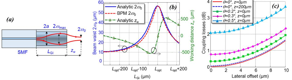
**Fig. 1.** (a) Principle of the SMF-GIF microlens, (b) calculation of beam waist and working distance based on the analytical method and BPM method, and (c) calculation of 55  $\mu\text{m}$  beam waist coupling losses for different angular misalignments and axial gap related to lateral offset.
