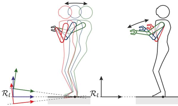
Fig. 3. Hands compensation experiment. Left: hands position is constant in  $\mathcal{R}$  whereas the floating-base moves. Right: hands position moves in  $\mathcal{R}_l$  whereas the floating-base is fix.
