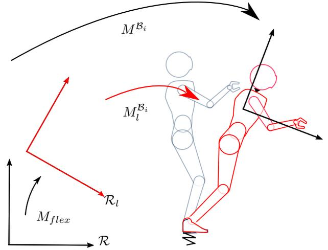
Fig. 2. Definition of the frames used for the modeling of the dynamics of the flexibility.  $M_l^{\mathcal{B}_i}$  is the position of the body  $\mathcal{B}_i$  in the rigid-body control frame  $\mathcal{R}_l$ .  $M^{\mathcal{B}_i}$  is the position of the same body  $\mathcal{B}_i$  in the world reference frame  $\mathcal{R}$ .  $M_{flex}$  is the homogeneous matrix between these two frames.
