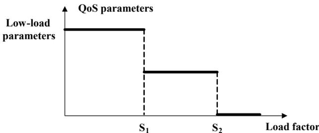
Fig. 3. QoS parameters reduction using the staircase policy
