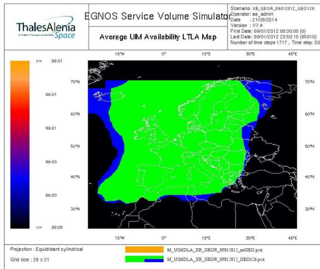
Figure 13: APV1 service area with/without GEO Ranging
