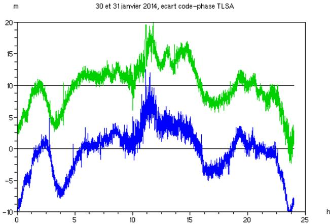
**Figure 7: code-phase for PRN 120 in Toulouse, 30 and 31<sup>st</sup> January 2014**
