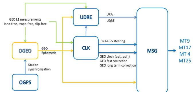
Figure 4: GEO orbit and messages generation processing
