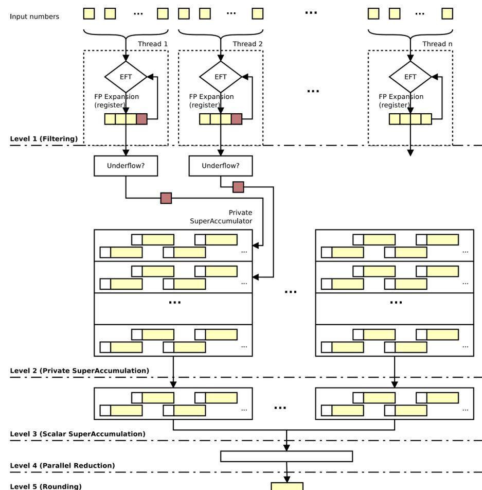
Fig. 1: Hierarchical superaccumulation scheme.
