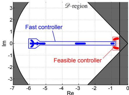
Fig. 6. Closed-loop poles for all the *discretized-P<sub>2</sub>* systems with 0.5 mm step on  $\delta$
