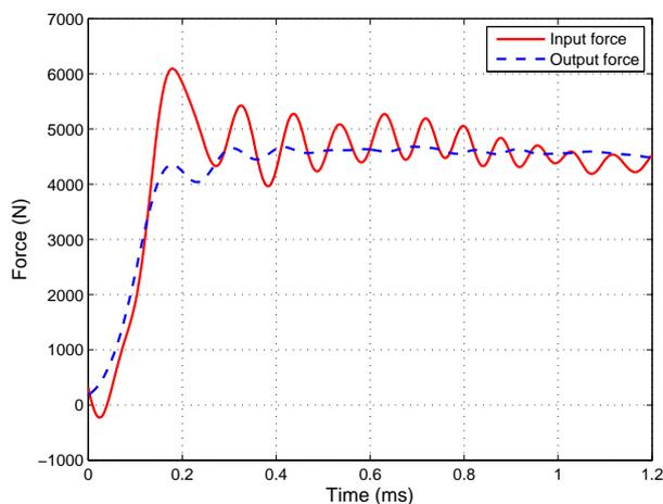
Figure 2: Forces history at specimen interfaces for a test at 10  $m/s$ . Force equilibrium is checked.
