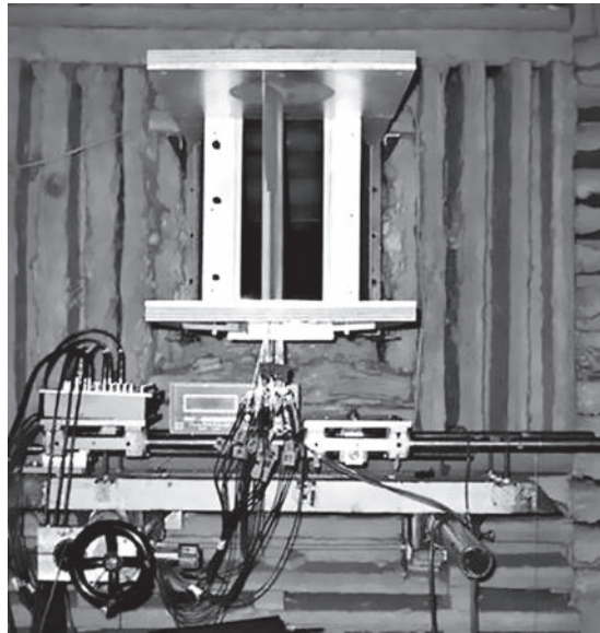
Figure 4: Picture of ECL facility showing the narrow nozzle flow and the horizontal end-plates.
