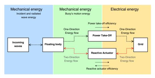
Fig. 2. Energy flow from the waves to the grid.
