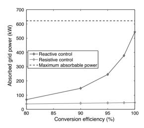
**Fig. 9.** Mean annual absorbed power at l'Ile d'Yeu under various conversion efficiency, France.
