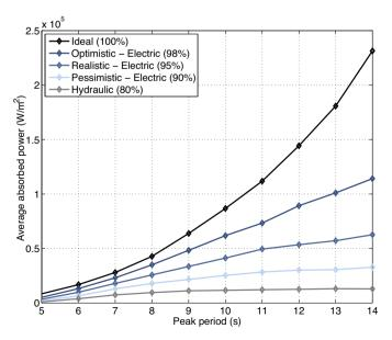
**Fig. 6.** Grid power as a function of spectrum peak period (irregular waves) without control and with control with different actuators efficiencies.
