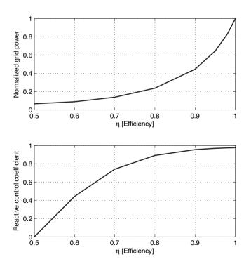
$\textbf{Fig. 4.} \ \, \textbf{Grid power and optimal reactive control coefficient as a function of actuators efficiency in a 9 s regular wave with 1 m wave amplitude.$
