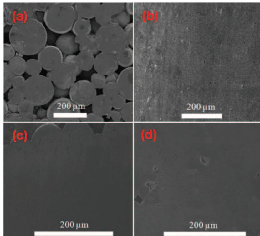
*a* as received powder sintered at 1250°C for 2 h via RHS; *b* 4 h ball milled powder sintered at 1250°C for 2 h via RHS; *c* as received powder sintered via SPS with completion of shrinkage at 860°C during continuous heating; *d* core region of 4 h ball milled powder sintered at 1250°C for 30 min via MWS
