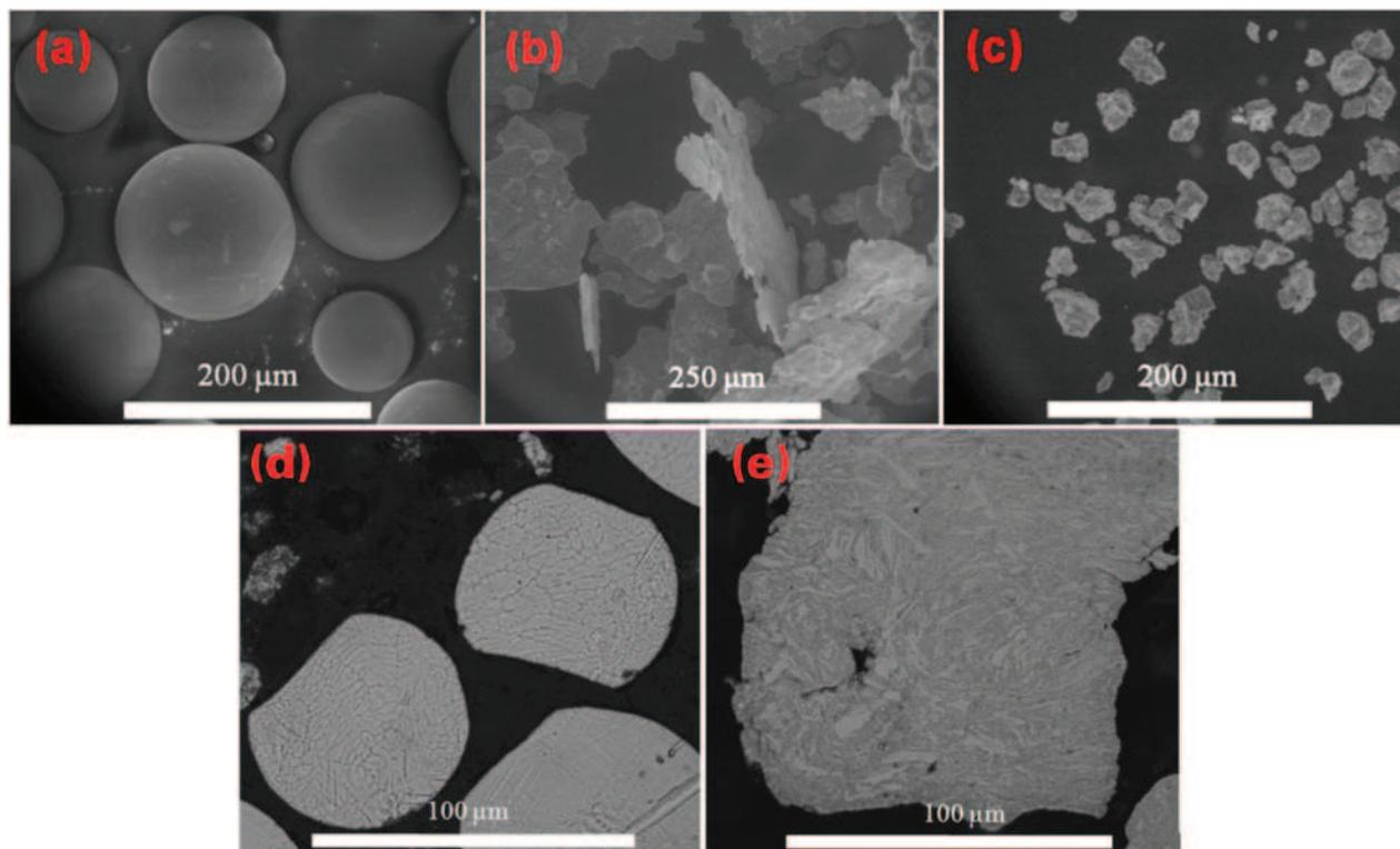
a as received; b ball milled for 1 h; c ball milled for 4 h; d etched cross-section of as received; e etched cross-section of ball milled for 4 h
