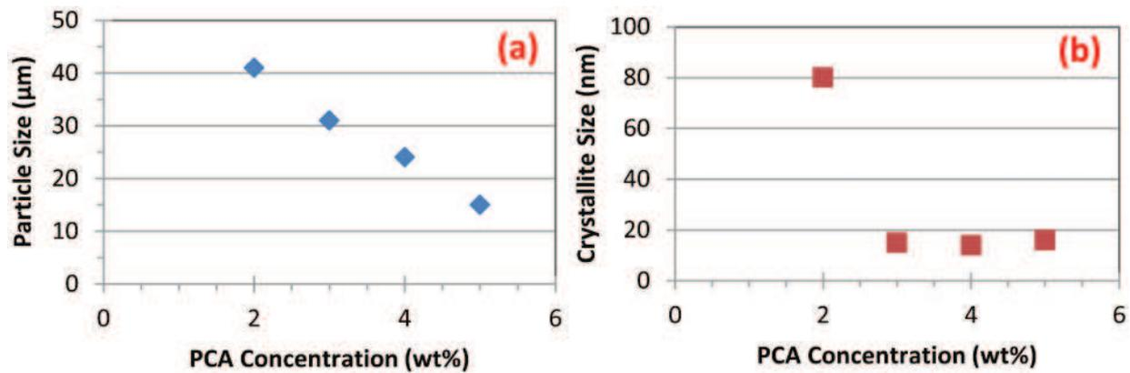
4 *a* average particle size (via SEM image analysis) and *b* average crystallite size [via XRD analysis of (002) reflection] of Ti-6Al-4V powder ball milled for 4 h as function of PCA concentration
