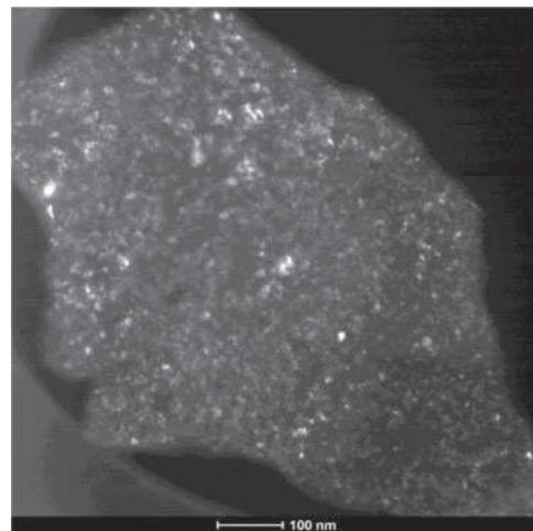
3 Dark field TEM image of Ti-6-4 powder ball milled for 4 h with presence of 4 wt-% stearic acid
