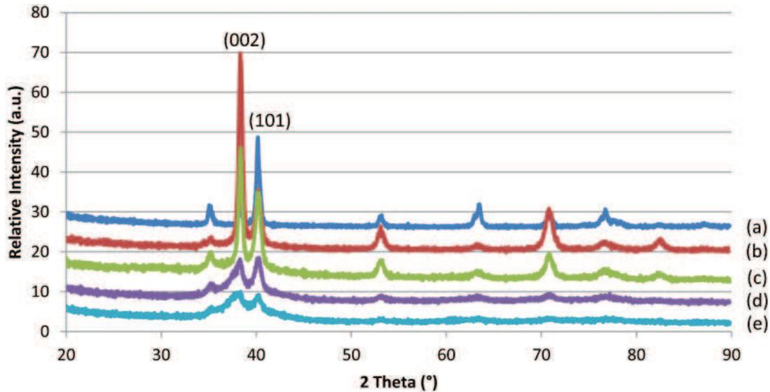
a as received; b ball milled for 1 h; c ball milled for 2 h; d ball milled for 3 h; e ball milled for 4 h (all are with 4 wt-% stearic acid)
