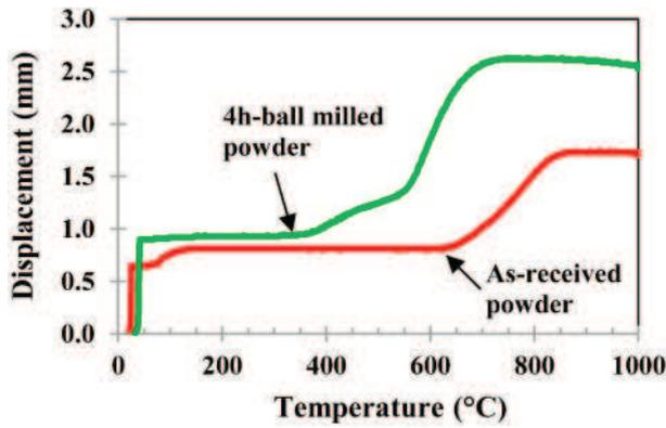
**6 Punch displacement curves during SPS with heating rate of 100°C min<sup>-1</sup>; arrows point to onset temperature for shrinkage during continuous heating for powder compacts indicated**
