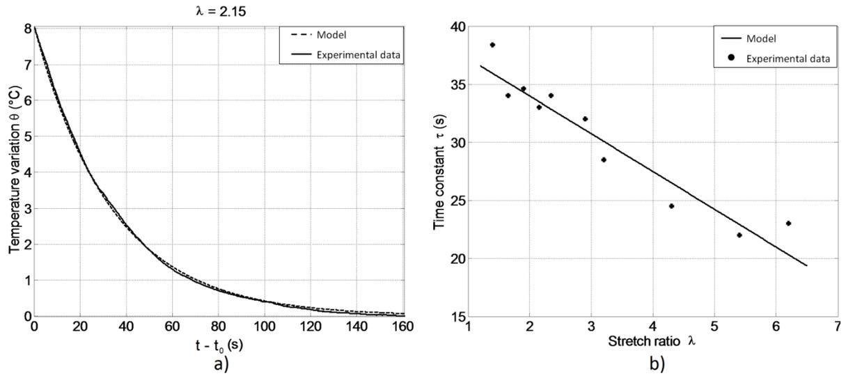
Figure 2: Identification of the time constant  $\tau$  characterizing the heat exchanges with the outside of the specimen. Left: example of natural return to ambient temperature, for the specimen stretched at  $\lambda = 2.15$ . Right: values of  $\tau$  as a function of  $\lambda$ .
