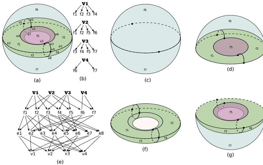
Figure 8: (a) A representation of a subdivision  $C^d$  made of four volumes. (b) The faces incident to each volume. The boundary of volume **V1** (resp. **V2**, **V3**, **V4**) is represented in (f) (resp. (d), (g), (c)). The incidence graph of  $C^d$  is represented in (e).
