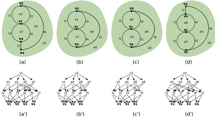
Figure 9: A regular  $CW$ -complex  $C$ , which dual is represented in Fig. 8.  $C$  is made of four volumes  $v_1..v_4$ , eight faces  $e_1..e_8$ , seven edges  $f_1..f_7$  and four vertices  $\mathbf{V}_1.. \mathbf{V}_4$ . On (a) – (d), the boundaries of volumes  $v_1, v_2, v_3, v_4$  ; on (a') – (d'), the corresponding incidence graphs.
