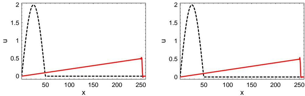
Figure 13: Propagation of an initial localized pulse using the LW3 scheme with artificial viscosity at time  $t = 500$  (i.e. the front has propagated along 500 mesh sizes). a)  $\Delta t = 0.2$ ; b)  $\Delta t = 0.5$
