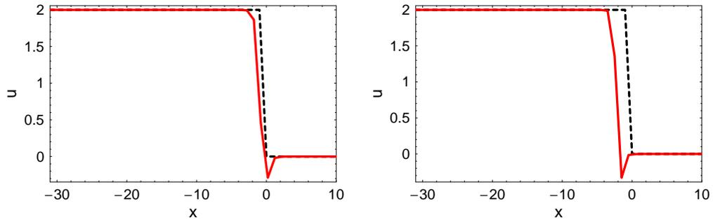
Figure 8: Propagation of an initial abrupt front using the WB scheme with artificial viscosity at time  $t = 500$  (i.e. the front has propagated along 500 mesh sizes). a)  $\Delta t = 0.2$ ; b)  $\Delta t = 0.5$ .
