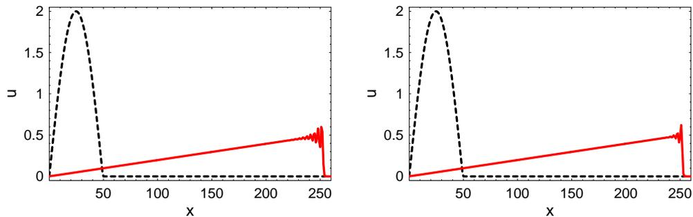
Figure 6: Propagation of an initial localized pulse using the LW scheme with artificial viscosity at time  $t = 500$  (i.e. the front has propagated along 500 mesh sizes). a)  $\Delta t = 0.2$ ; b)  $\Delta t = 0.5$
