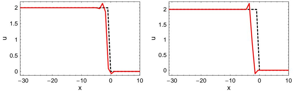
Figure 12: Propagation of an initial abrupt front using the LW3 scheme with artificial viscosity at time  $t = 500$  (i.e. the front has propagated along 500 mesh sizes). a)  $\Delta t = 0.2$ ; b)  $\Delta t = 0.5$
