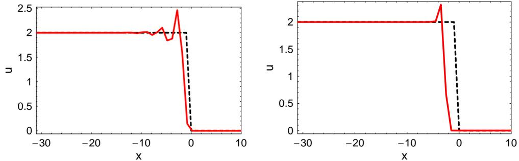
Figure 5: Propagation of an initial abrupt front using the LW scheme with artificial viscosity at time  $t = 500$  (i.e. the front has propagated along 500 mesh sizes). a)  $\Delta t = 0.2$ ; b)  $\Delta t = 0.5$
