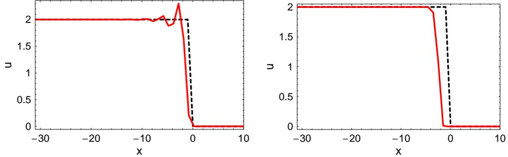
Figure 10: Propagation of an initial abrupt front using the Mac-Cormack scheme with artificial viscosity at time  $t = 500$  (i.e. the front has propagated along 500 mesh sizes). a)  $\Delta t = 0.2$ ; b)  $\Delta t = 0.5$ .
