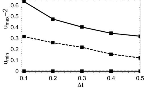
Figure 7: Variations of minimum and maximum of the shock vs temporal step for the LW scheme:  $u_{max} - 2$  varies between upper solid line and dotted line, while lower solid line corresponds to  $u_{min}$ .
