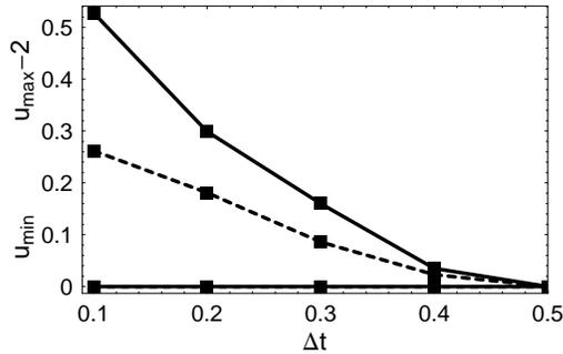
Figure 11: Variations of minimum and maximum of the shock vs temporal step for the MC scheme:  $u_{max-2}$  varies between upper solid line and dotted line while lower solid line corresponds to  $u_{min}$ .
