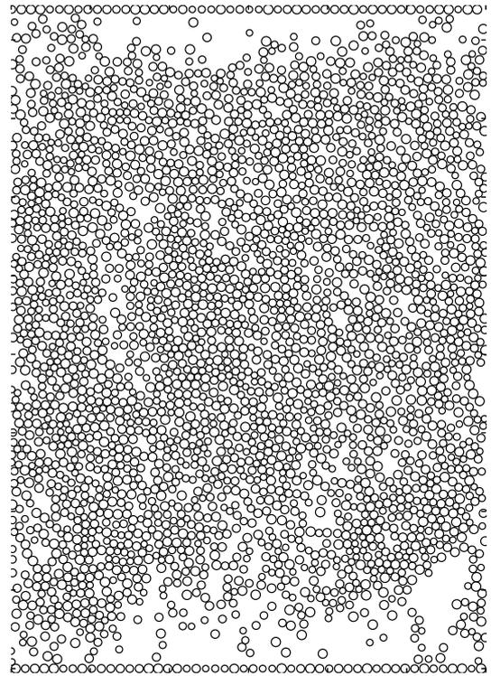
FIG. 1: Snapshot of the simulated system. A 2D granular material is sheared between two bumpy walls. The lower wall is fixed, the upper one moves horizontally at a constant velocity  $V_{top} = 100$  and is submitted to a constant vertical stress  $P = 1$ .
