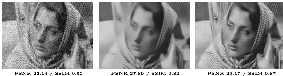
Fig. 3. (left) Noisy image f = u_0 + w , (center) nonlocal-means u^* , (right) debaised \tilde{u}^* .
