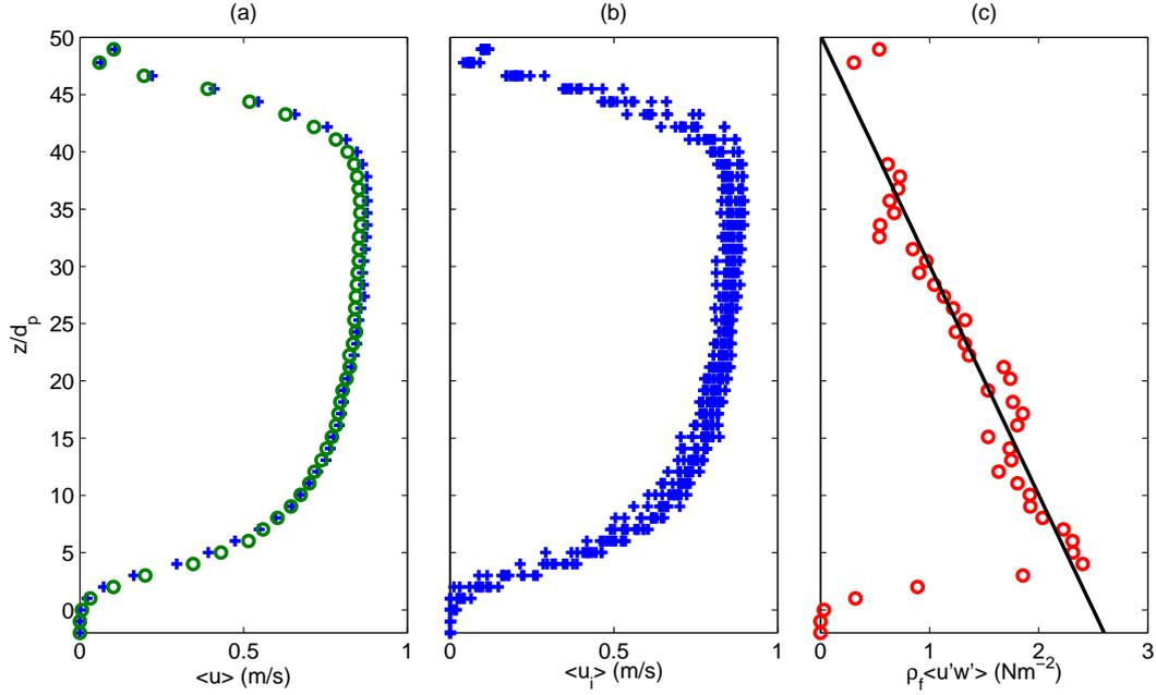
FIGURE 6. (a) Mean streamwise velocity profiles averaged over  $t \in [40 - 43]$ s (+) and over  $t \in [43 - 46]$ s (o). (b) Mean streamwise velocity profiles averaged over  $t \in [40 - 46]$ s for the 11 realisations. (c) Absolute Reynolds shear stress  $\rho_f \langle u'w' \rangle$  (o) and linear fit (—).
