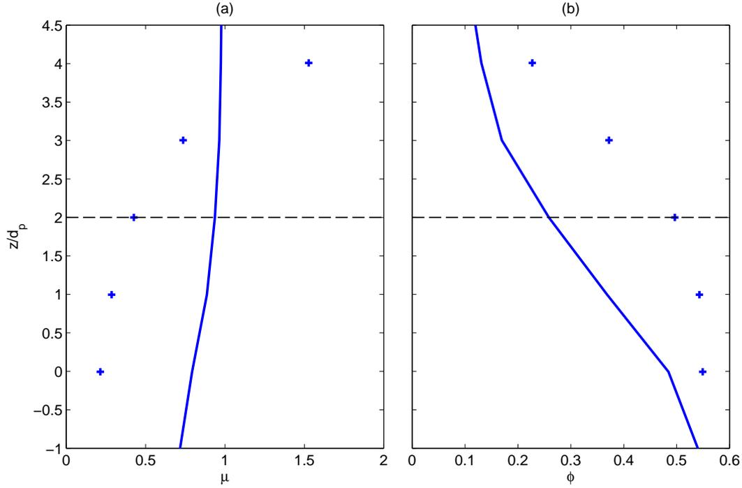
FIGURE 12. Comparison between measurements (+) and prediction from the granular rheology  $\mu(I)/\phi(I)$  (—) for the friction coefficient profile (a) and the concentration profile (b). The horizontal dashed line represents the position for which  $I = 1$ .
