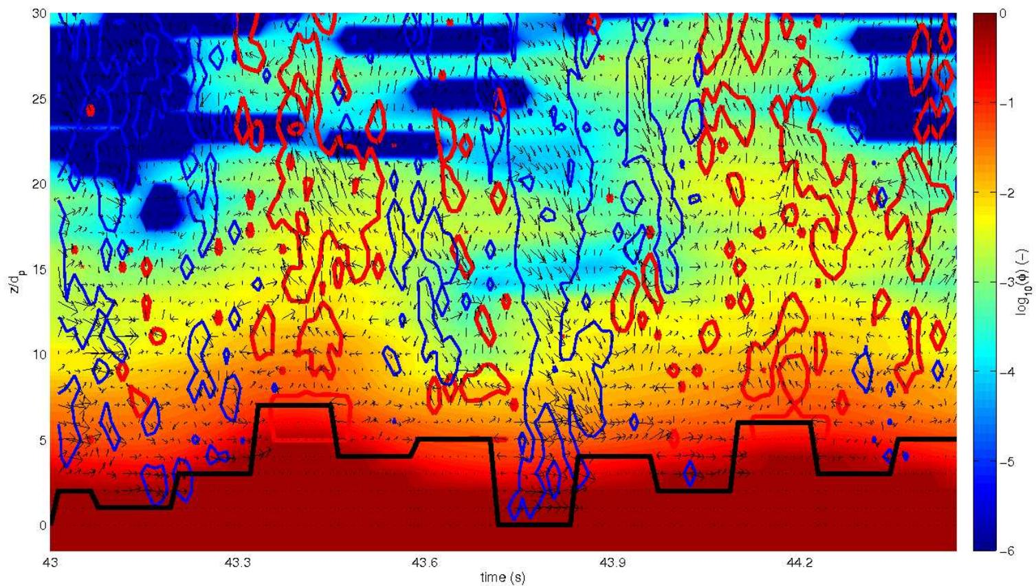
FIGURE 13. Time evolution of the measured bed interface position (black thick line) and concentration measurements (colorplot in base 10 logarithm) associated to coherent structures detection: the red and blue contours represent the ejections and sweeps respectively as iso-contours of  $H = 2$  as evaluated in Mignot *et al.* (2009). The vector plot represents the instantaneous 2C velocity fluctuations.
