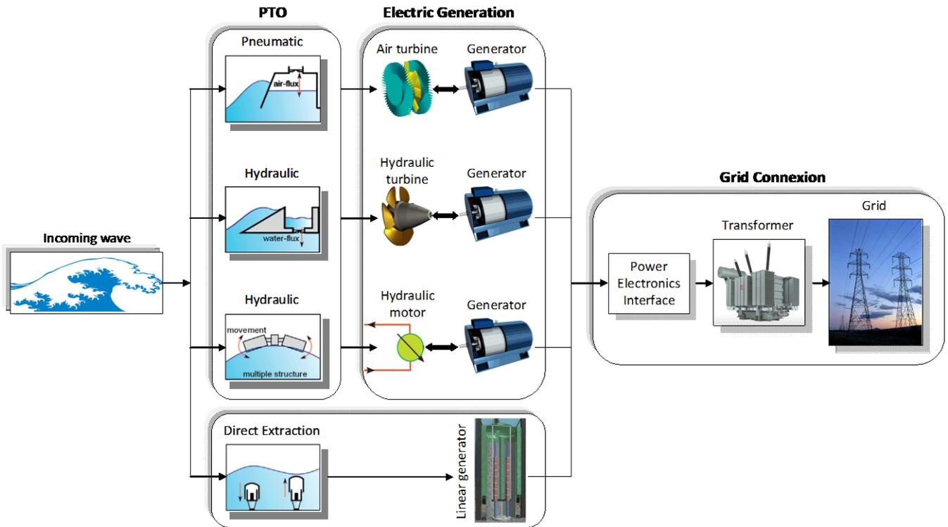
Fig. 7. WEC different type of conversions.
