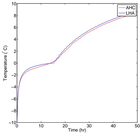
Figure 18: Comparison between the temperature history at  $x = 5$  cm obtained by the LHA (Number of subdivision= 5 and  $N_{basic} = 80$ ) and the one obtained by the AHC ( $\Delta T = 0.5^\circ C$  and  $N_{basic} = 320$ )
