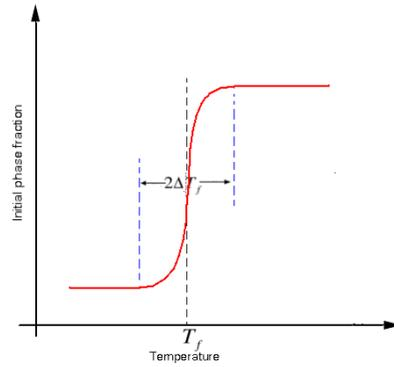
Figure 12: Approximation of the initial phase fraction over a small temperature interval according to the error functions.
