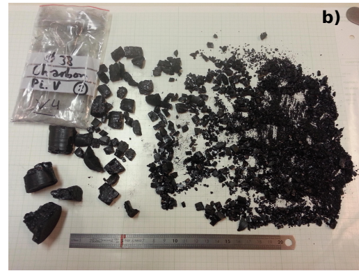
Coal failed under simple compression
