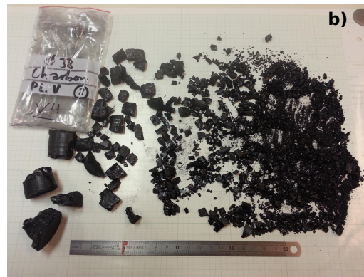
Coal failed under simple compression
