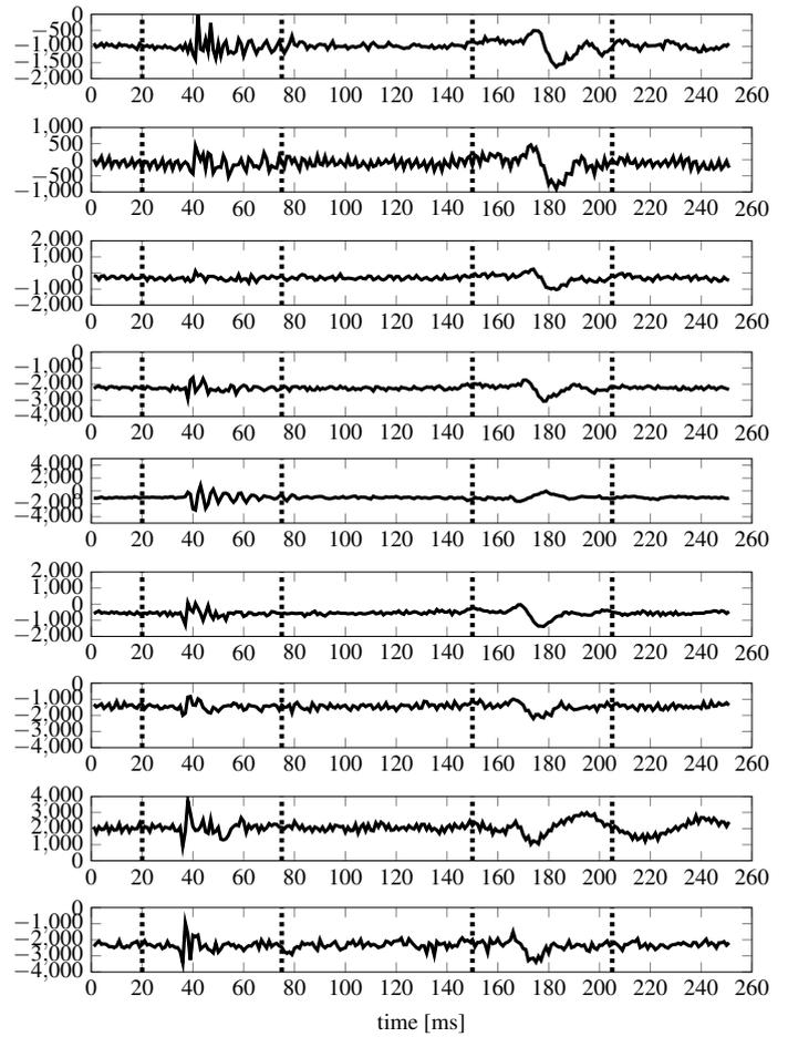
Figure 7: Example of an event from the Argentière glacier - 2012: record from the array with distinct P and S waves - vertical component
