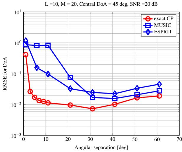
Figure 3: RMSE [rad] vs angular separation [deg] - endfire perspective
