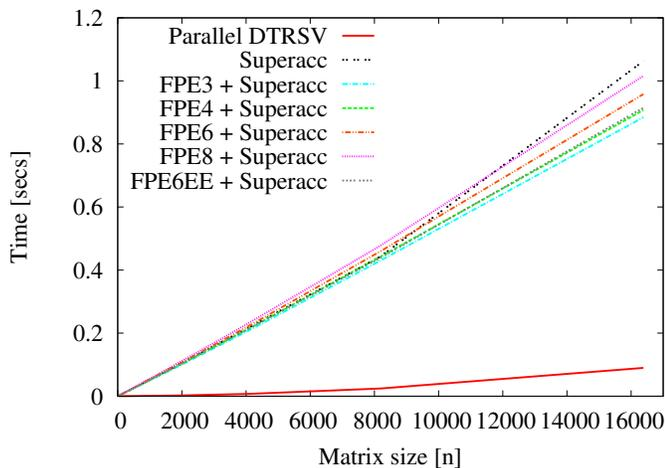
Fig. 5: Performance of substitution algorithms on NVIDIA K5000.
