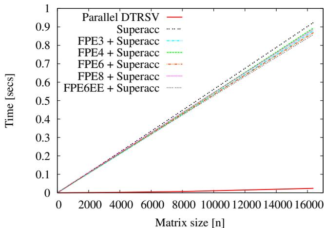
Fig. 4: Performance of substitution algorithms on NVIDIA K20c.
