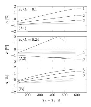
Figure 6: Amplification rate  $\alpha$  of the three first modes of the engines versus the temperature gradient imposed for the three configurations (A1), (A2), and (B). Modes 4 to 6 are also given in gray. A positive amplification rate means that a wave at the frequency of the corresponding mode will be amplified by the TAC.  $\alpha=0$  for mode 1 represents the onset threshold, for which  $T_h-T_c=\Delta T_o$ .
